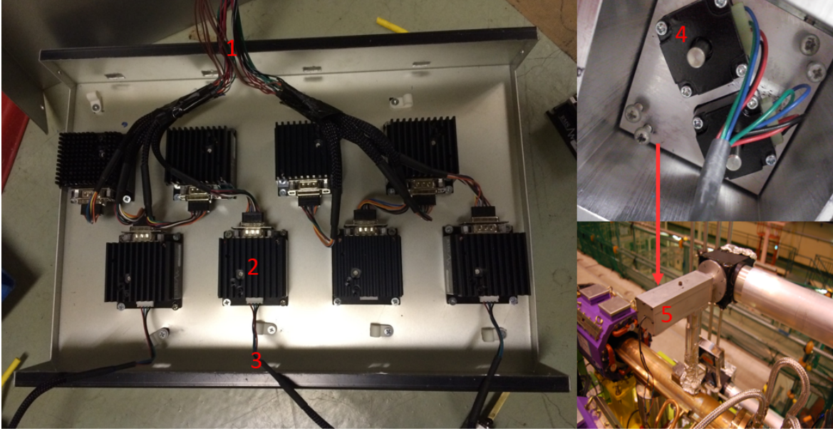
Figure 3.22: Remotely controlled mirrors: 1)Input cable from the computer to the motor drivers; 2)Motor drivers; 3)Output cable from the motor drivers to the stepper motors; 4)Stepper motor inside the primary elbow; 5)Primary elbow.
