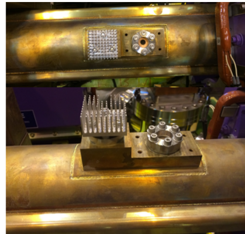
Figure 3.6: Vacuum mirror design on the left; top and side view of the heat sink and beam pipe window on the right.
