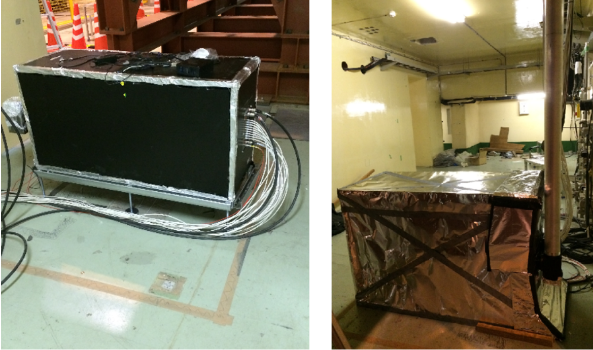
Figure 3.20: The optical box, shown without covering on the left, and with covering on the right.
